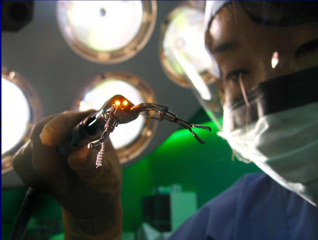
The tip of the endoscopic robot (two arm type)
