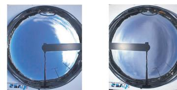
Figure 4 sky image showing piranometer overestimation of cloud coverage, point A in the graphic, due to clouds spatial distribution.
