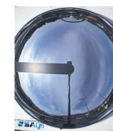
Figure 5 sky image showing piranometer underestimation of cloud coverage, point B in the graphic, due to low sensitivity to thin clouds.
